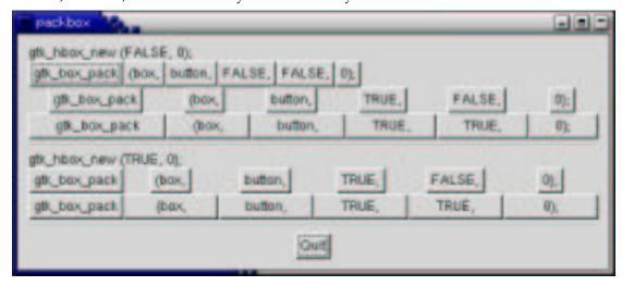
Each line contains one horizontal box (hbox) with several buttons. The call to gtk\_box\_pack is shorthand for the call to pack each of the buttons into the hbox. Each of the buttons is packed into the hbox the same way (i.e., same arguments to the gtk\_box\_pack\_start() function).
